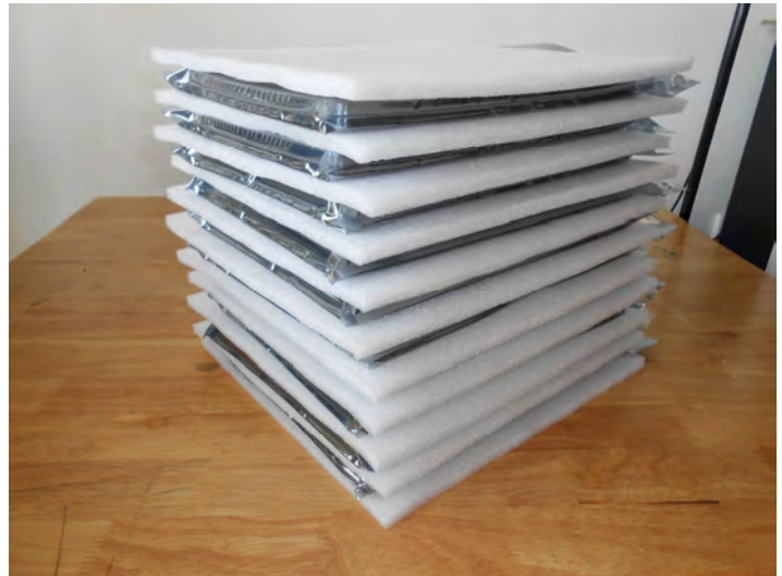
Foam Sheets are Slightly Larger than Trays
